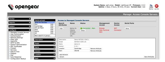
Click **Show** in the **Serial Ports** column of any particular *Managed Console Server* to view all devices attached to the serial ports of that *Managed Console Server*
