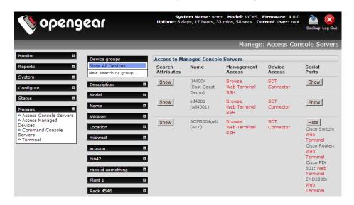
Where configured you can then click Web Terminal to connect to the device on the remote Managed Console Server's serial port - as a terminal
