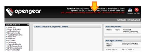
➤ Click **Web Terminal** to connect to the *Managed Console Server's* command line. The Web Terminal service uses AJAX to enable the web browser to connect through the *CMS* to the *Managed Console Server* using HTTPS as a terminal.
