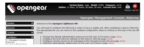
**Note** The default username / password is *root / default*. However on the initial deployment during the load process you will be prompted to enter and confirm a new root password. If you simply have upgraded to a new version you won't be prompted for a new root password, the device will just boot normally with the password it already has.
