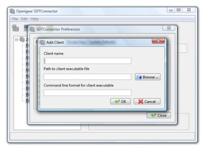
Enter a **Name** for the client. Enter the **Path** to the executable file for the client (or click **Browse** to locate the executable)
